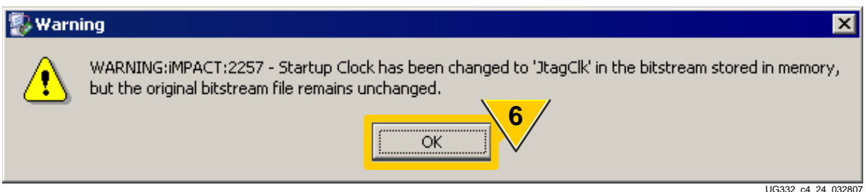
Figure 12-13: iMPACT Uses the JTAG Clock Input TCK for Startup Clock when Programming via JTAG
